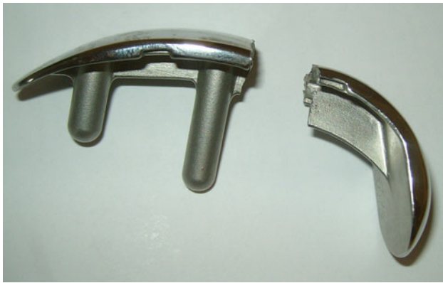
Fig. 1 Fracture of the posterior aspect of the femoral implant adjacent to the peg
