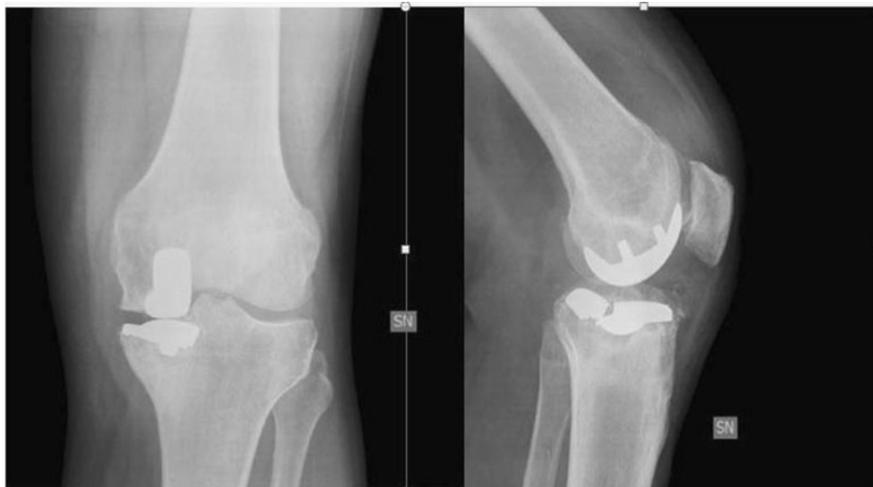
Fig. 3 Fracture of a CrCoMo tibial component with bone loss
